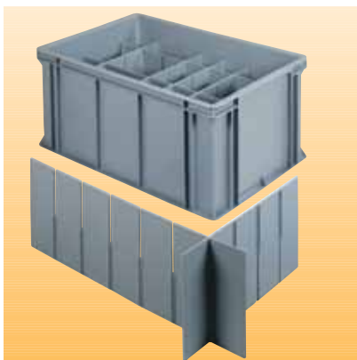
Divider 3620 and 5620, height 200 mm, smallest division 71 x 80 mm, suits containers 600 x 400 mm.
