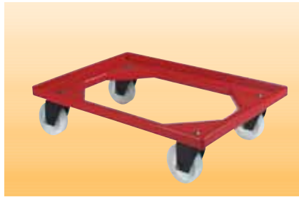
Plastic trolley, red Size 600 x 400 mm, with 4 plastic casters 100 mm dia. Max. load 250 kg Order No. 60.6400.004.000
